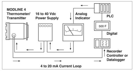
Modline 4 two-wire transmitter diagram
